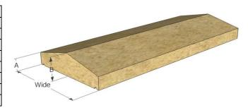
Coping - weathered two ways, typically used on boundary and garden walls. This design allows rain water to 'run-off' both sides of the wall.
